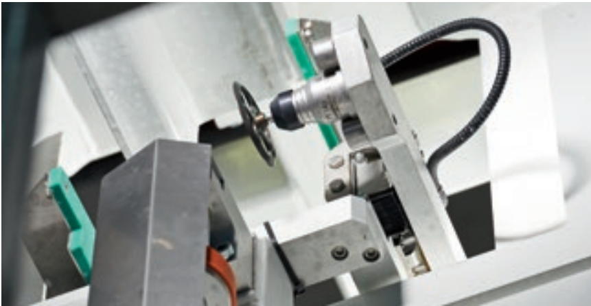
Diamond grinding wheel and polishing wheel presetter.
