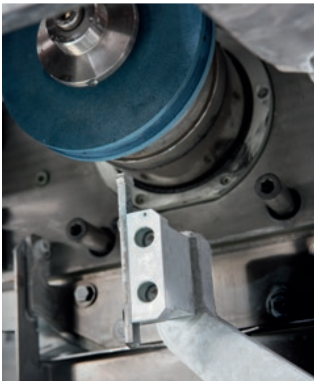
Diamond grinding wheel and polishing wheel presetter.
