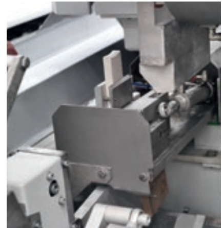
Three-position stick dresser for profiling and shaping diamond wheels.
